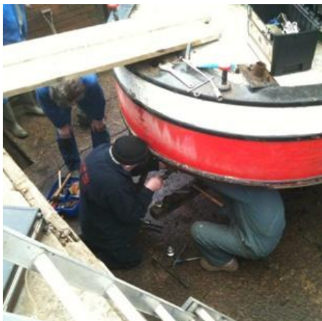
The prop shaft being replaced (left) and in place (right).
