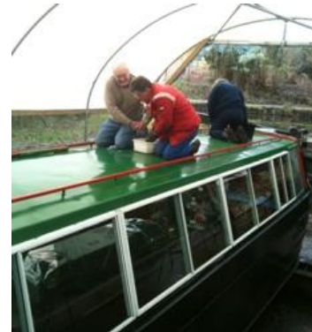
Cleaning of the John Pinkerton under way in the Deepcut dry dock. Among other jobs done this year the hull was pressure washed and repainted, and the rest of the bodywork was cleaned and touched up.
