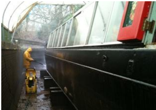
Cleaning of the John Pinkerton under way in the Deepcut dry dock. Among other jobs done this year the hull was pressure washed and repainted, and the rest of the bodywork was cleaned and touched up.
