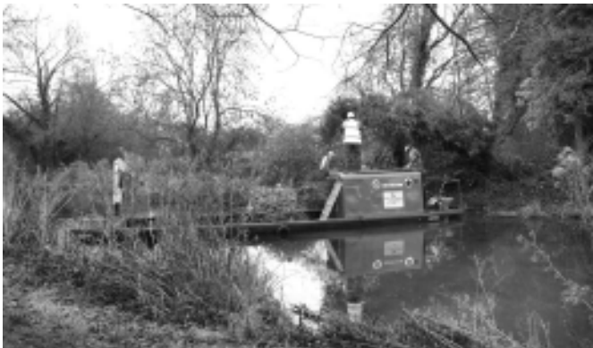
Left: The work boat's cabin roof makes a useful work platform for tree pruning at North Warnborough.
