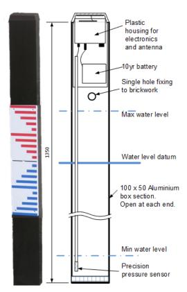
The SCP uses Internet-of-Things (IOT) technology to provide 24/7 displays of water level and related data history to Rangers' smartphones or office PCs, measured by special sensors at strategic canal locations. Actions can then be taken accordingly. The BCA & BCS have been working with a Surrey-based start-up company to develop these cutting-edge facilities that hopefully can then be sold worldwide and provide us with a small 'benefit share' of resulting sales.
