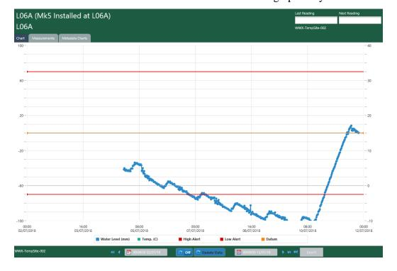
The depth of water is indicated on the Y axis (+/-100mm, or 4 inches, in this case). The falling part of the graph in this example (indicating a level drop) shows what would appear if a leak had been taking place over several days (e.g. due to an open lock paddle) with back-pumping also in operation, which accounts for the partial level recovery ("stepping") each day. The subsequent sharp rise reflects the return to datum level once the situation has been rectified.
